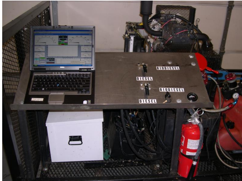
Figure 2. Mobile biodiesel demonstration unit used in ASBEP.
